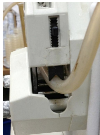
Tubing threaded through the teeth of the pump
