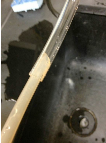
Insert nozzle tubing into distilled H 2 O tubing
