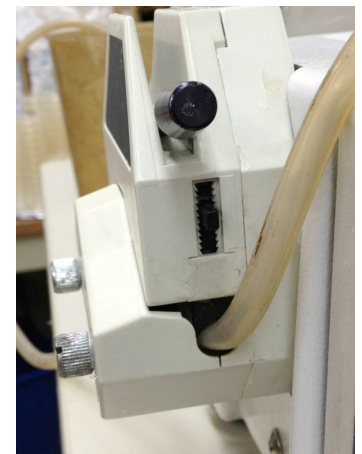
Tubing closed in the pump
